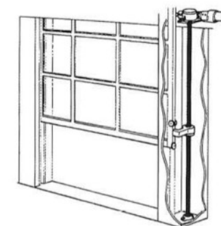
Automatic switch on large windows (doors)
